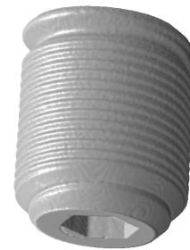
Figure 1.8: 3D rendering of the thresholded volumetric image of a dental implant.
