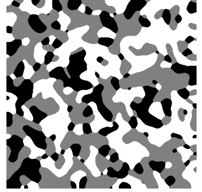
Figure 1.3: Image of a segmented fuel cell with three phases. Black represents air, grey is cathode, and white is anode.
